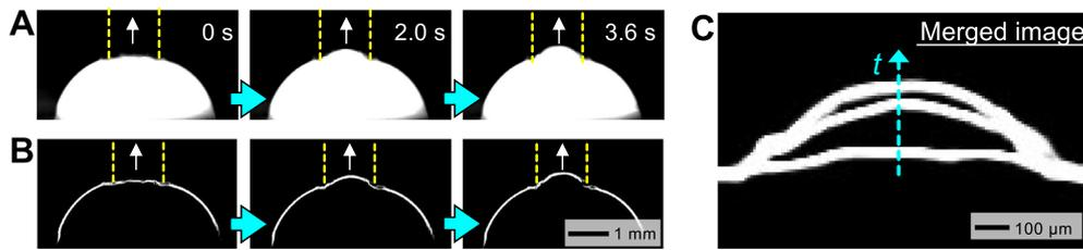
**Fig. 2.** Gelatin hydrogel (4%w/v) used to evaluate functionality of the measurement system: (A) Stiffness measurement was demonstrated using a dome-shaped 4% w/v gelatin hydrogel formed on a PDMS substrate. To enhance visibility of gel deformation, fluorescein dye was added to the gelatin. (B) Via edge detection, the deformed shape of the gelatin was determined. (C) Merged image of the deformed region of the gelatin showing elongation of the gel due to vacuum pressure over time.
