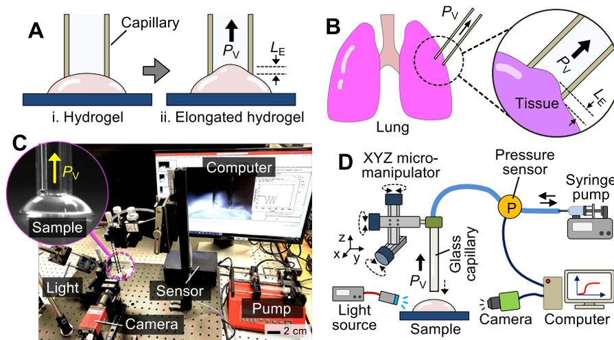
**Fig. 1.** Overview of vacuum-based measurement of elastic moduli of soft biomaterials, including hydrogels and tissues: Schematic of (A) hydrogel and (B) lung tissue deformed via vacuum pressure.  $P_V$ : vacuum pressure.  $L_E$ : elongation length. (C) Custom-built system to measure the stiffness of soft biomaterials and *ex vivo* lung. (D) Schematic of measurement system. P: Air pressure sensor.
